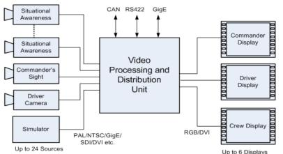
Full qualification including gun shock Multi-channel high speed >20GB bandwidth digital switch
